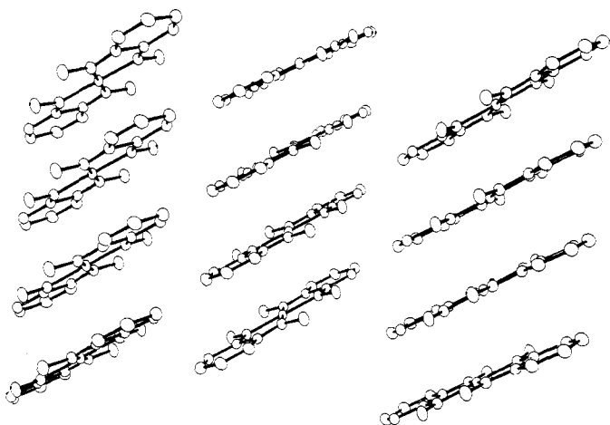
Figure 6. Packing diagram of Ni(bqd) 2 plotted from the data of ref 9. Vibrational ellipsoids are drawn at the 50% level.
